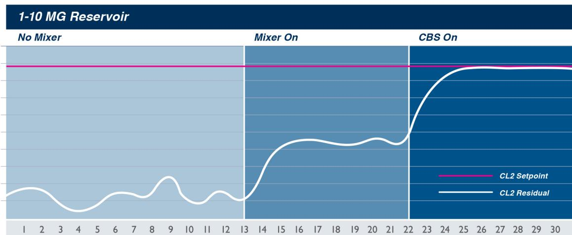
Uncirculated reservoirs tend to have low residuals throughout the reservoir, especially at the upper levels. When reservoirs are circulated, the residual tends to be higher and uniform throughout the entire reservoir. The Chloramine Boosting System allows the operator to set an ideal residual level throughout the entire reservoir.
